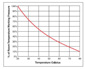
Example from the Celsius Chart If Working Pressure at 20°C is 14 bar, then the WP at 50°C is  $14 \times 40\%$ , or 5.6 bar.
